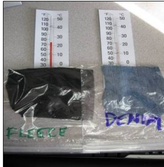
Figure 1: Bags with Insulation placed over thermometers
