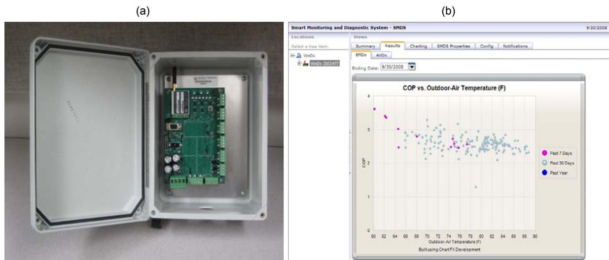
**Figure I: SMDS (a) Hardware and (b) User Interface Window Showing Air-Conditioning COP Versus Outdoor-Air Temperature.**
