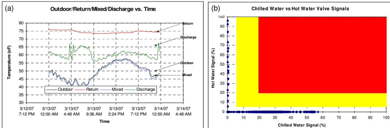
**Figure B: (a) Improperly Operating Economizer and (b) Properly Operating Chilled- and Hot-Water Valves**
