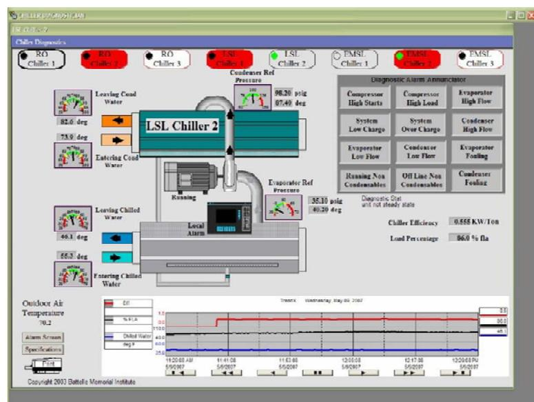
**Figure H: User Interface of an Automated Centrifugal Chiller Diagnostician.**
