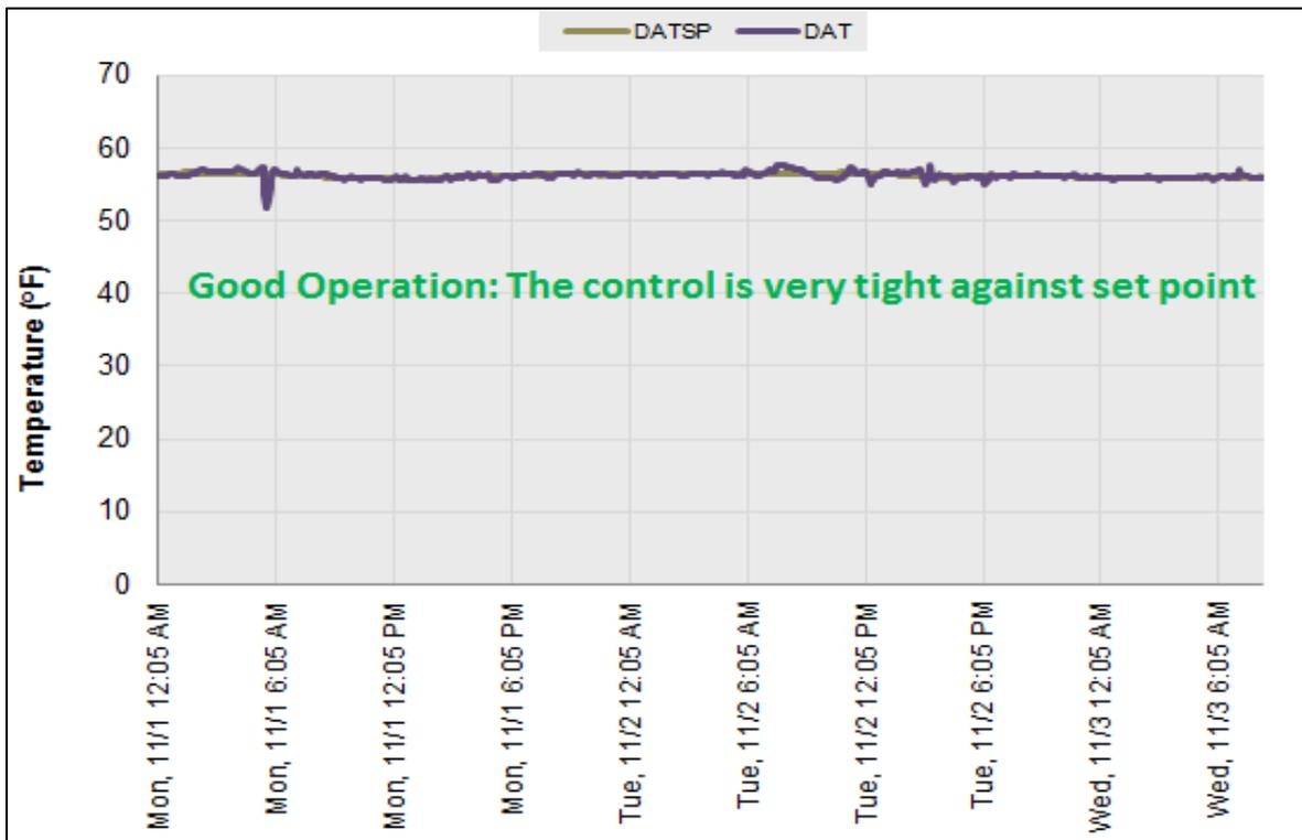
Figure 8: Discharge-air temperature very steady against the set point.
