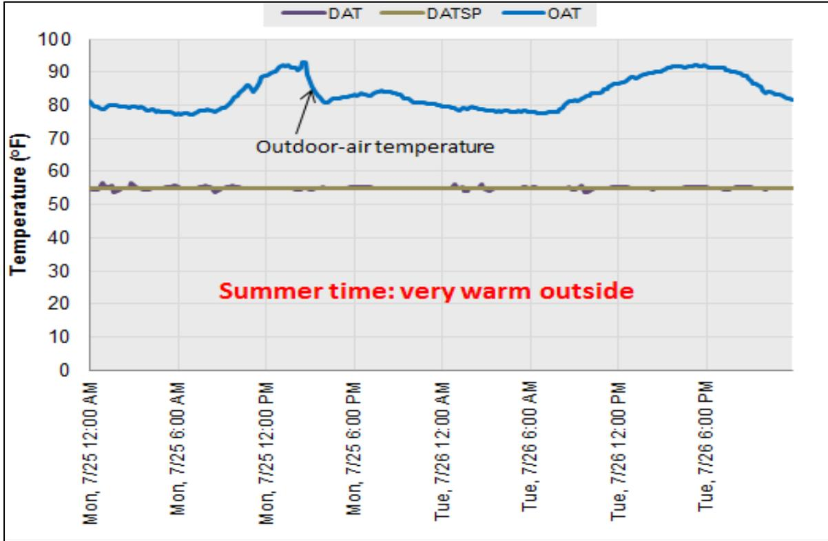
Figure 5: Discharge-air temperature and set point for an air handler.
