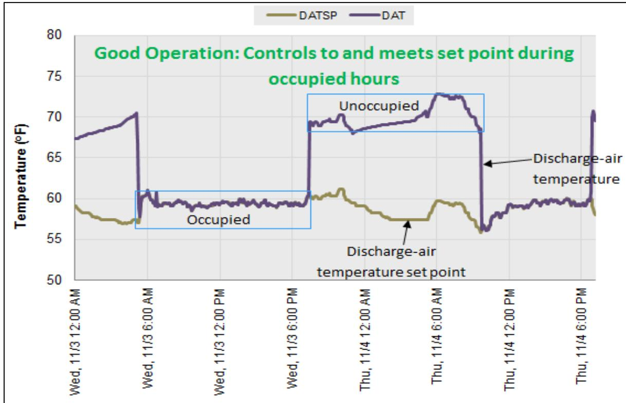
Figure 4: Discharge-air temperature controls to set point very well.
