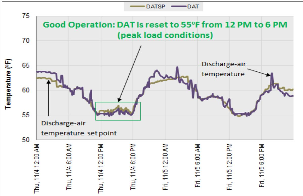
Figure 2: Air-handler with good discharge-air reset-schedule.
