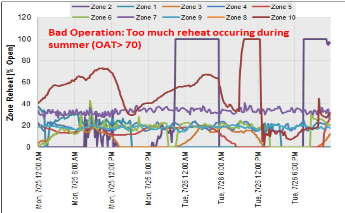
Figure 6: Reheat valve signals vs. time for zones served by AHU in Figure 5.
