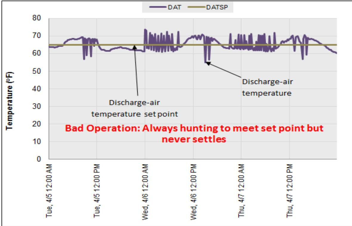
Figure 7: Unstable discharge-air temperature.
