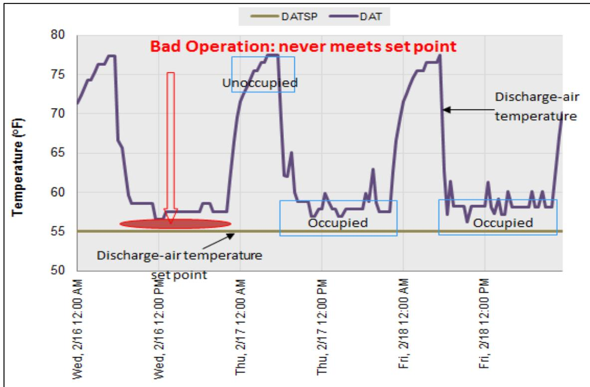
Figure 3: Discharge-air temperature never meets set point.
