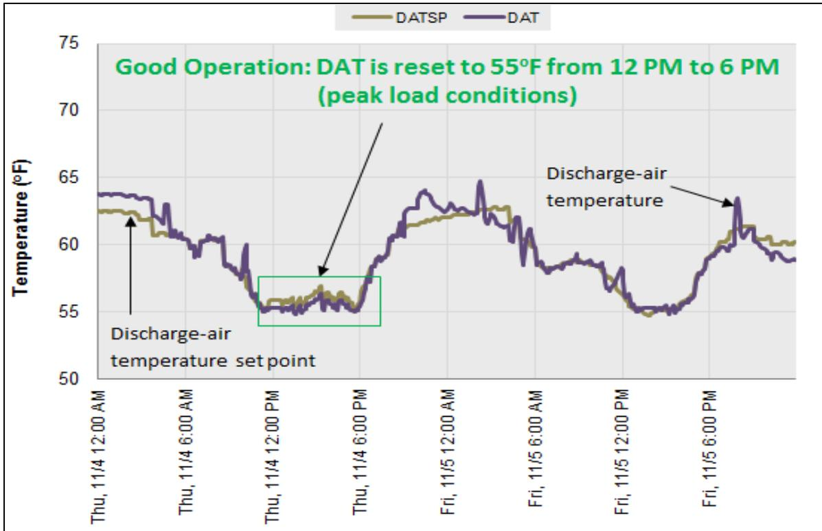
Figure 2: Air-handler with good discharge-air reset-schedule.
