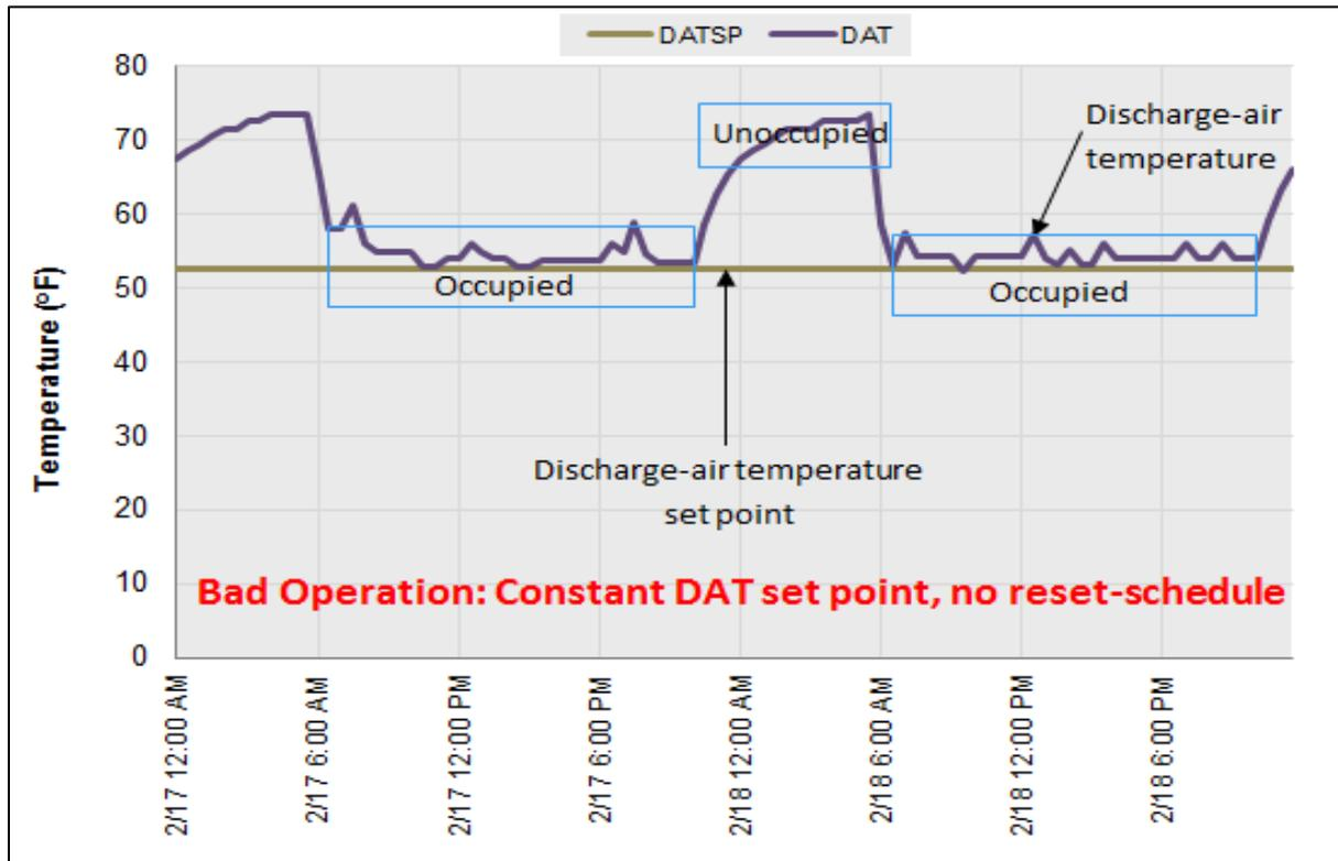
Figure 1: No discharge-air reset-schedule in place.
