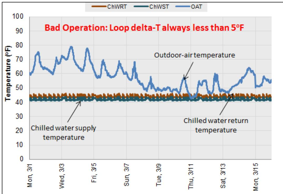
Figure 5: Example of bad operation, where the loop delta-T is less than 5°F, indicating too low chilled water supply temperature set point.
