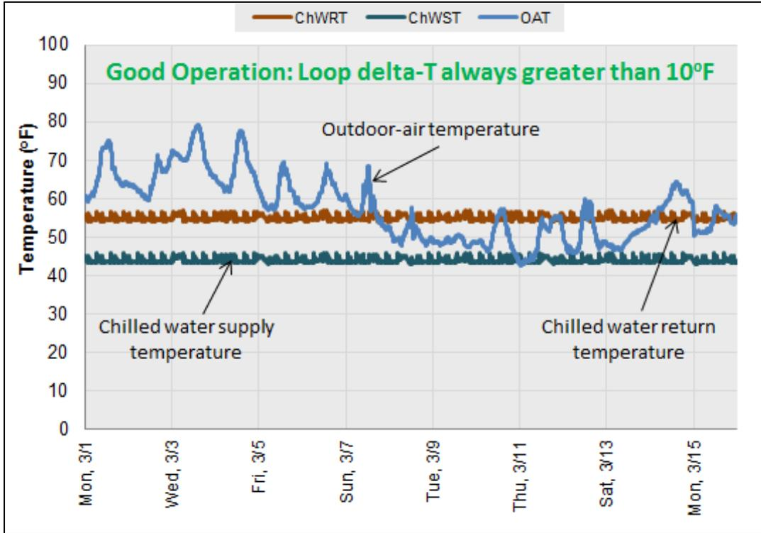
Figure 6: Example of good operation, where the chilled water supply temperature set point is higher for similar outdoor conditions as in Figure 5, thus increasing the loop delta-T to the design conditions.
