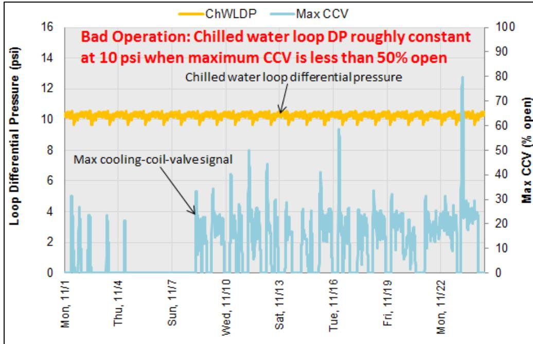
Figure 7: Example of bad operation, where the loop differential pressure is not reset when the maximum cooling-coil-valve signal is always less than 50% open.
