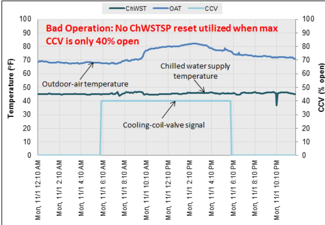
Figure 3: Example of bad operation, where the cooling-coil-valve signal only indicates 40% open and the chilled water supply temperature set point remains unchanged.
