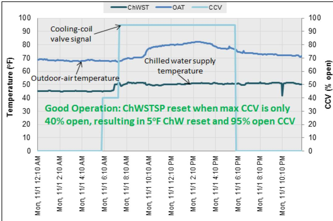
Figure 4: Example of good operation, where the chilled water supply temperature set point is reset by 5°F, and the cooling-coil-valve signal responds by opening 95%.
