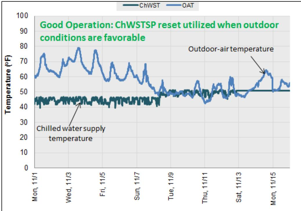
**Figure 2: Example of good operation, where the chilled water supply temperature set point is reset when the outdoor conditions are favorable.**
