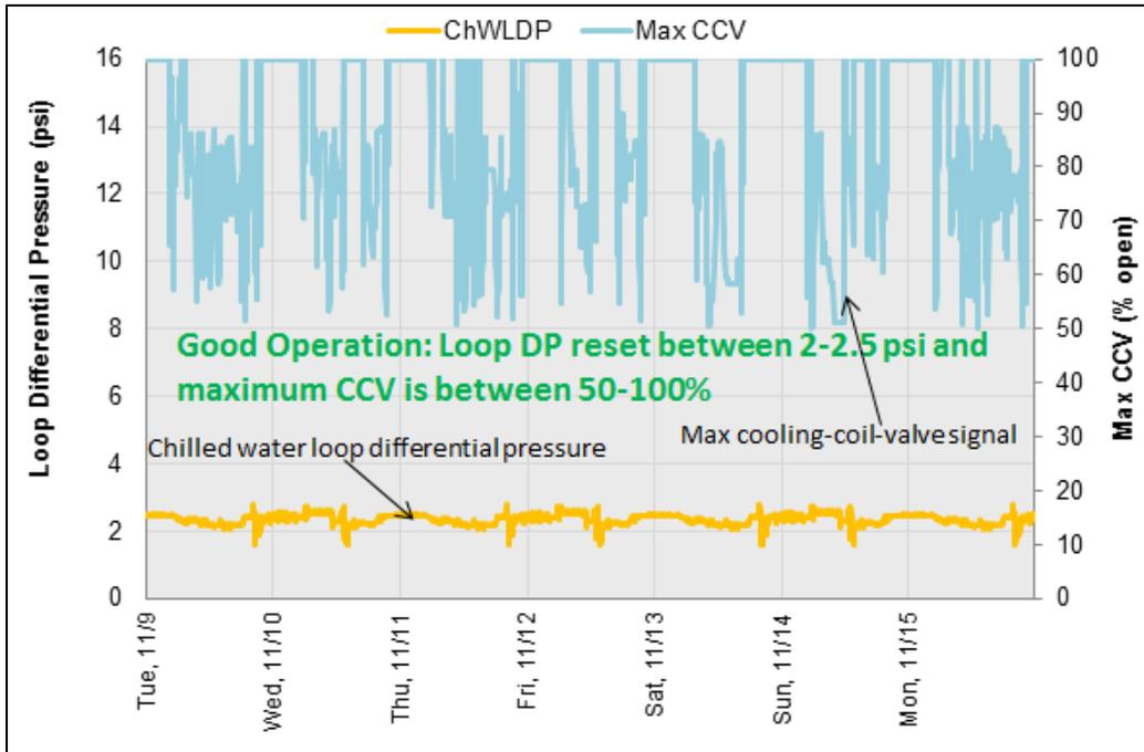
**Figure 8: Example of good operation, where the loop differential pressure is reset between 2 and 2.5 psi while the maximum cooling-coil-valve signal is between 50% and 100% open.**
