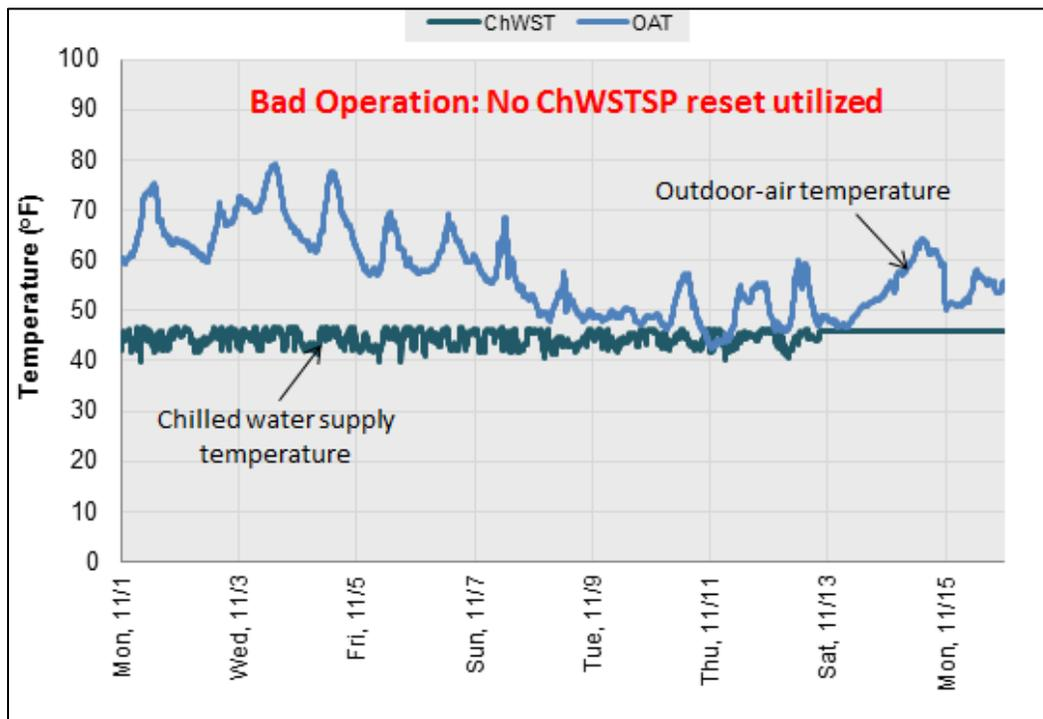
Figure 1: Example of bad operation, when the chilled water supply temperature set point is not reset during advantageous outdoor conditions (i.e., OAT less than 60°F).
