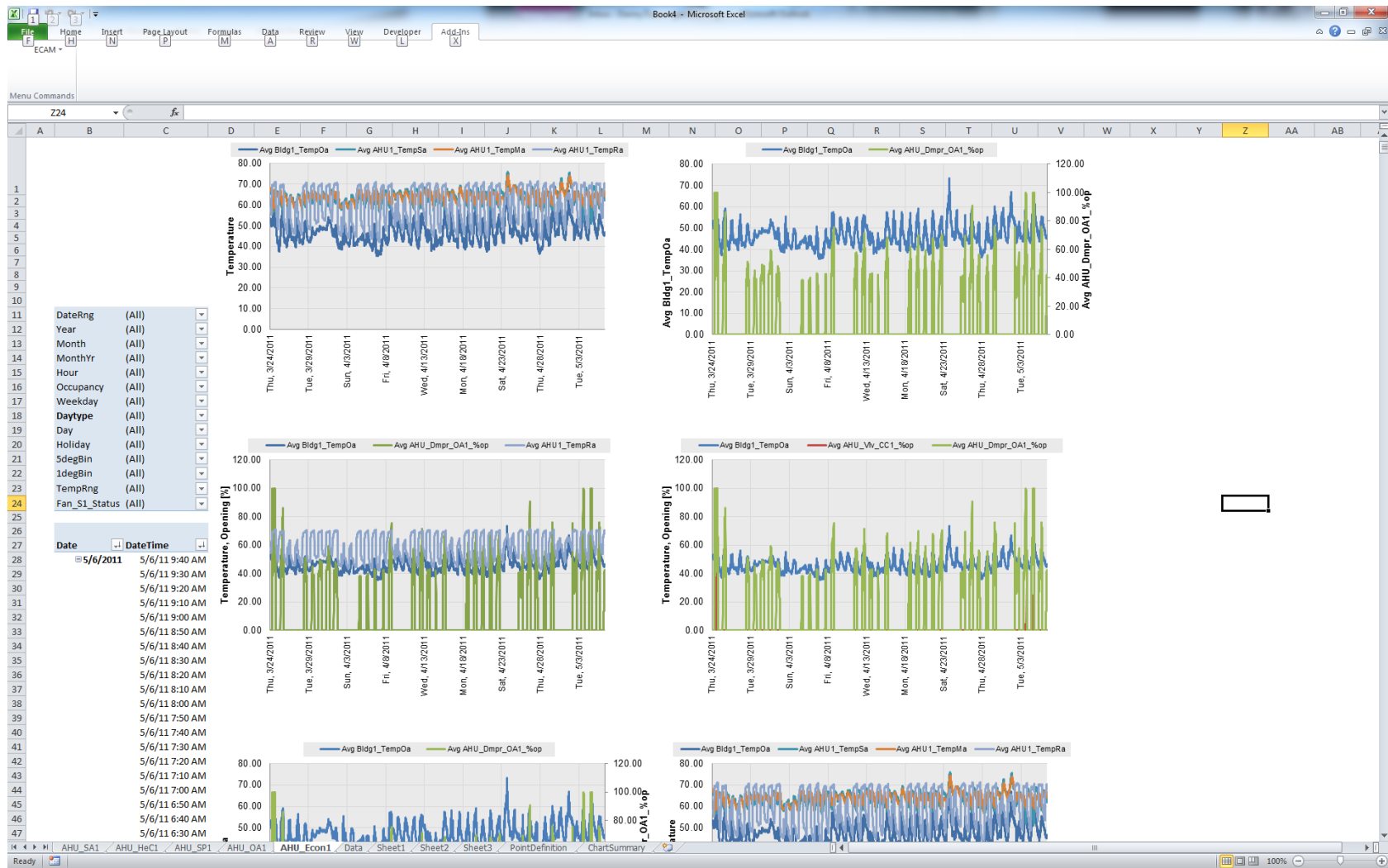
Figure 10-12: AHU charts in ECAM+ under the “PNL Re-Tuning” option. Here the AHU_Econ sheet is highlighted, but the user can see the other sheets that have been generated such as AHU_OA, AHU_SP, AHU_HeC, and AHU_SA.
